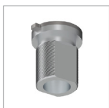
Retaining collar with male thread incl. smart slider for 360° rotation material: aluminium die cast for pendant rod M10 × 1 for pendant rod M13 × 1
